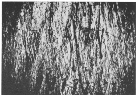
Figure 11 Micrograph of the tensile face of specimen 1 following four point bending. The wavy slip traces are due to \langle 011 \rangle slip on the maximum resolved shear stress plane which is near \{100\} . ( \times 45 ).
